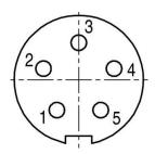
Connector Power supply and outputs
